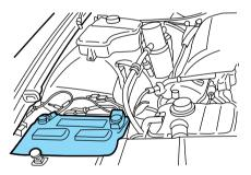
However, for severe usage or in high temperature climates, check the battery electrolyte level. Refer to the Scheduled Maintenance Guide for the service interval schedules.
